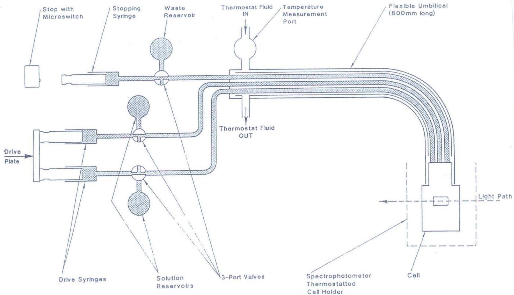
**Figure 1:** Schematic of the Hi-Tech SFA-20 Rapid Kinetics Accessory.
