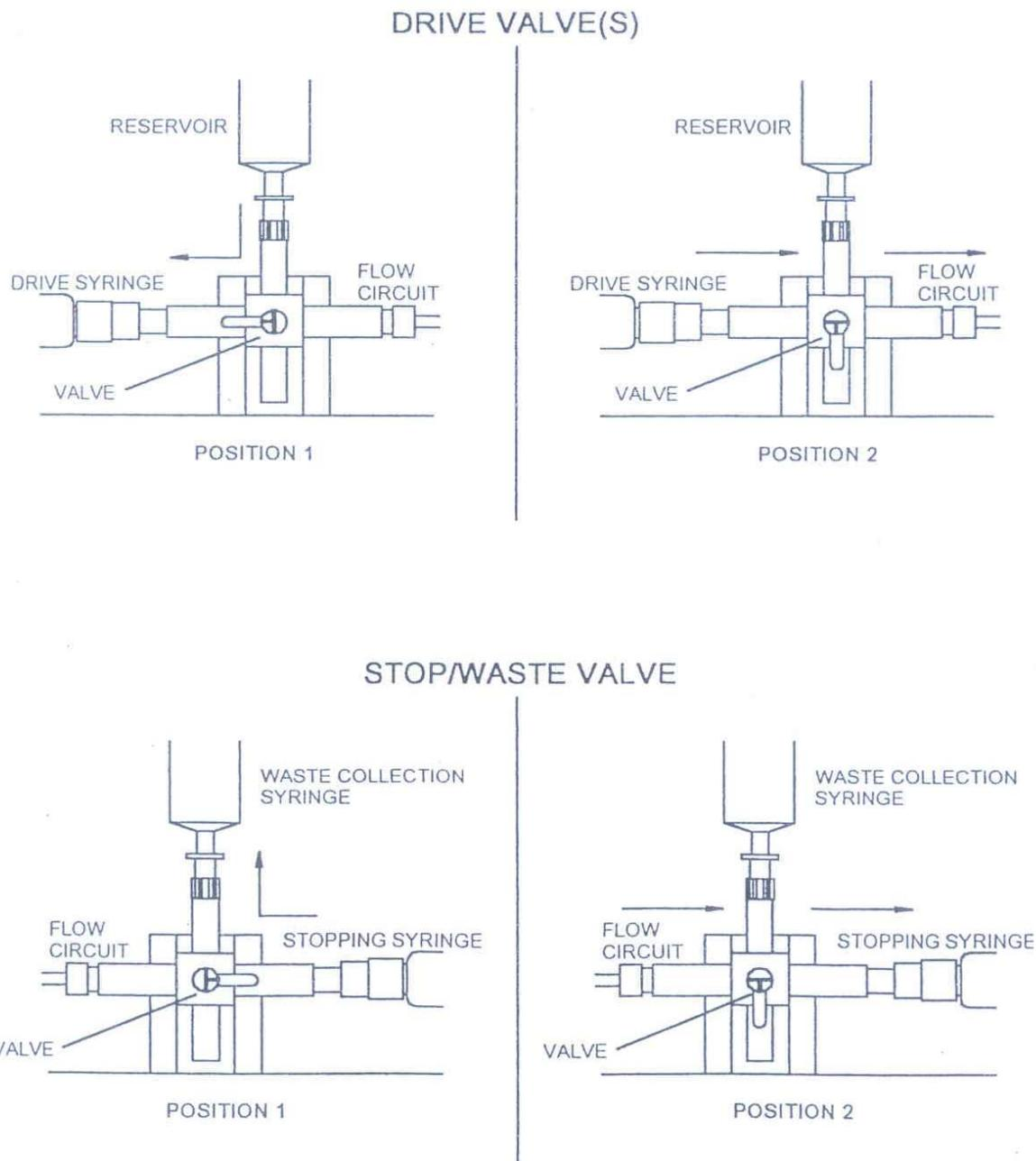
**Figure 2:** Valve positions on the Hi-Tech SFA-20 Rapid Kinetics Accessory.
